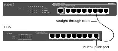
Figure 2-9 Connecting a hub to the Switch
